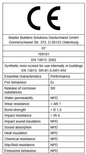
NPD = No Performance Determined. Performance determined in system build-up Master Seal Roof 2110
